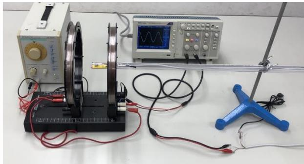
Fig. 4. Setup of Helmholtz coil experiment
