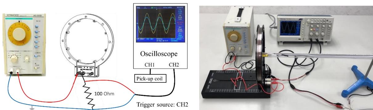
Fig. 3. Setup of pick-up coil experiment
