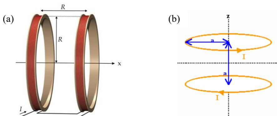
Fig. 1. Structure of (a) Helmholtz coil pair (b) Anti-Helmholtz coil pair
